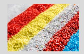
We stock a comprehensive range of different blast media for processing trials and maintain a large stock of standard media with different pellet sizes in our warehouse. The plastic de-flashing machines can be operated with the following media
